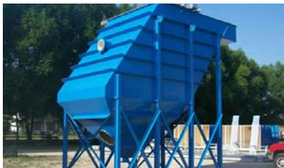
Inclined tube settlers are used in the lamella clarifier
